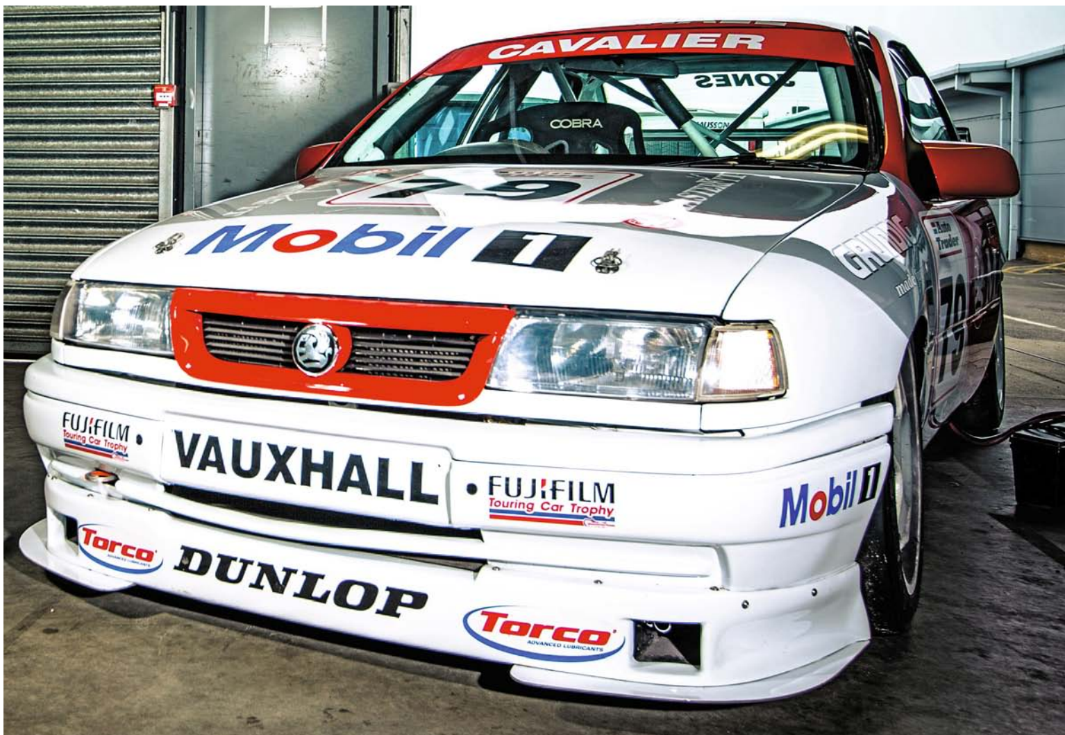
Ex-Allam Cavalier from 1994 now wears the splitter and wings introduced for '95. Reid reckons they improved the car but created less exciting racing thanks to increased difficulty in overtaking
