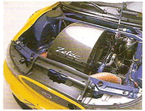
The V6 engine was not regarded as ideal and is buried deep under the scuttle with drive running through the vee
