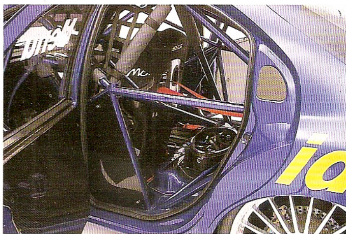
Mondeo's cockpit is very simple (top left) with floor mounted pedals and left hand drive to balance the weight of the engine. The rollcage (above) picks up on suspension mounts in the floor. Packaging the engine (left) was a problem, but Prodrive managed to reduce engine changing times from eight hours to one hour
